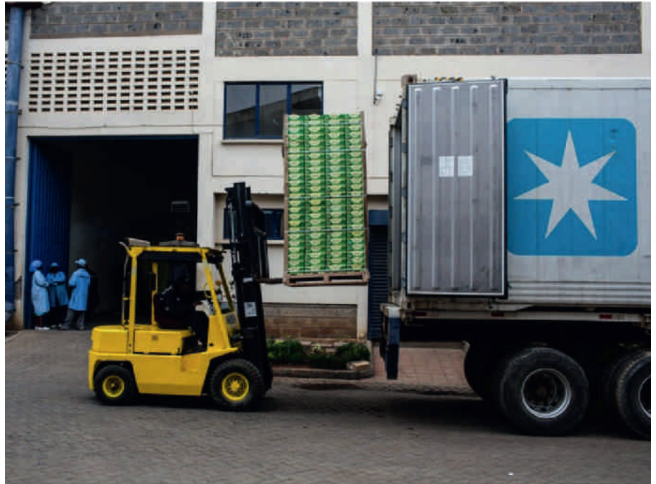
Figure 29: After Pre-cooling, Reefer Containers Are Packed Next to the Packing Facilities
